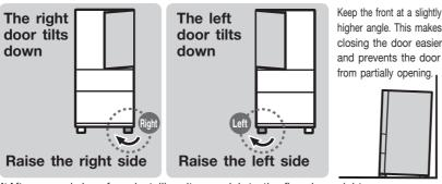
XAfter several days from installing, it may sink to the floor by weight. Please re-adjust the adjustable legs again.
